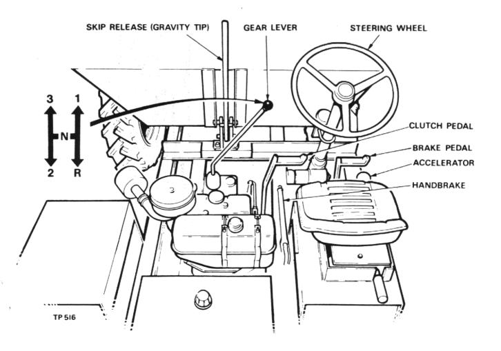
MACHINE SPECIFICATION FORWARD TIP SKIP (Gravity)
